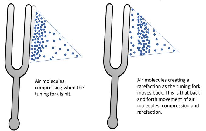
This tuning fork makes sound waves when struck which causes the vibrations (back and forth many times, called compression and rarefaction) as the vibrations slow and eventually stop, so do the sound waves that cause the vibrations and so does the sound.
